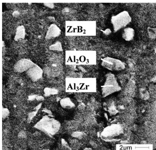
Fig. 4 Features of reinforced particles in the composites synthesized in Al-Zr-O-B system
